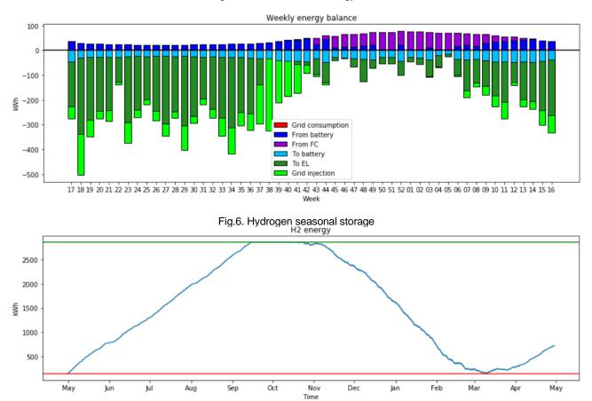
One can see that despite a short period when grid consumption was required during the commissioning of the system (fig. 4, month of May), the installation become self-sufficient. It proofs seasonal storage at residential scale by the use of hydrogen storage, supporting the penetration of RESs.
